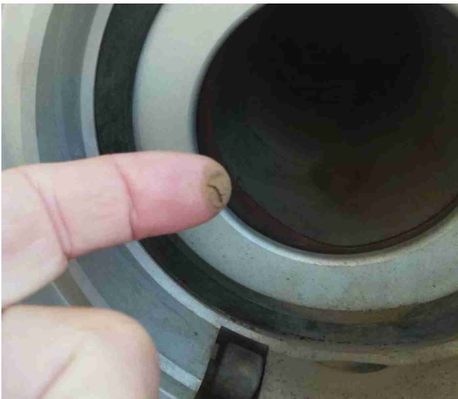
Moisture and dust particles will quickly cause damage to the injection parts of a diesel engine.
